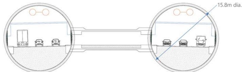
**FIGURE 8.3 - INDICATIVE DUAL 3 LANE BORED TUNNEL CROSS SECTION**
