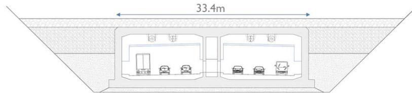
**FIGURE 8.4 - INDICATIVE DUAL 3 LANE IMMERSSED TUNNEL CROSS SECTION**
