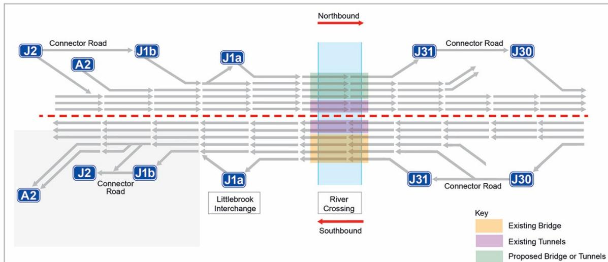
FIGURE 2.2 - ROUTE 1 SCHEMATIC LANE LAYOUT
