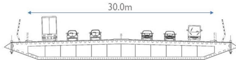
**FIGURE 8.2 - INDICATIVE DUAL 3 LANE BRIDGE CROSS SECTION**
