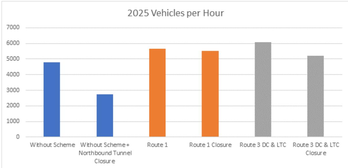
**FIGURE 4.14 - OFF-PEAK CROSSING FLOWS WITH AND WITHOUT A CLOSURE OF ONE OF THE DARTFORD TUNNELS IN 2025**
