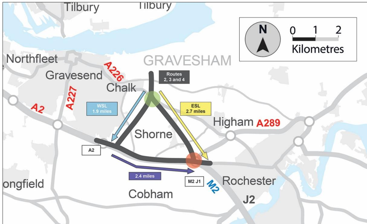
**FIGURE 4.12 - COMPARISON OF DISTANCES FOR TRAFFIC USING WESTERN SOUTHERN LINK AND EASTERN SOUTHERN LINK**
